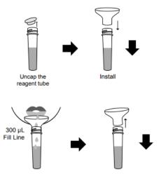
For individual Buffer Pack Unscrew the lid of an extraction reagent to open, add all of the extraction reagent into an extraction vial.
